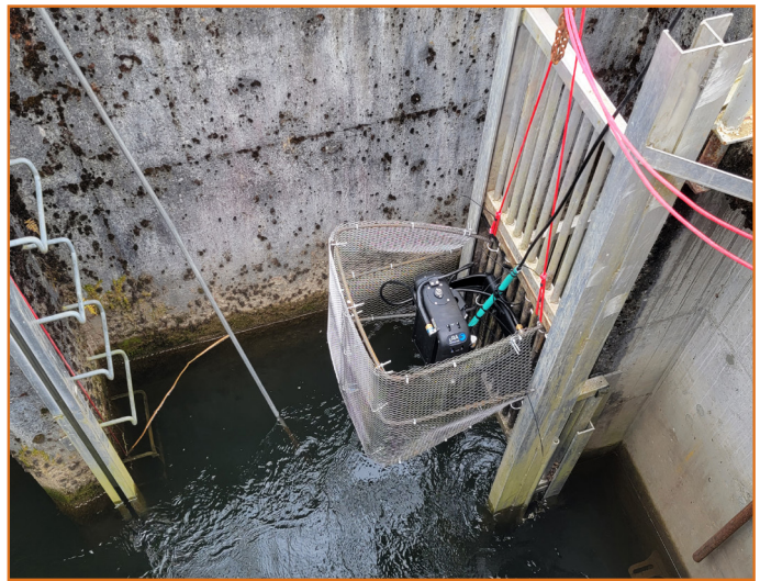
The Didson ARIS Imaging Sonar as it sits in the fish ladder at the Centralia Diversion Dam.
