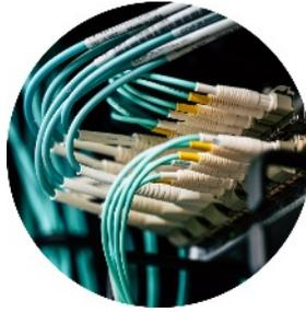
winding and has multiple bends? You could line the walls with mirrors and angle the light beam so that it bounces from side-to-side all along the hallway. This is exactly what happens inside an optical fiber line.
